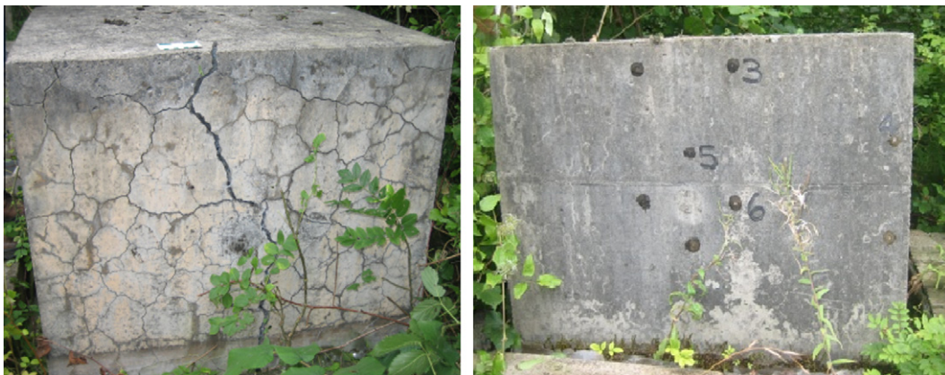
Fig. 6. Photographs of 18 year-old 915 mm blocks with TV sand on BRE exposure site block with 550 kg/m³ PC (left) and block with 450 kg/m³ PC + 150 kg/m³ FF fly ash (right).
