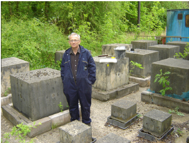
Fig. 1. View of BRE exposure site showing 915 mm blocks and 350 mm cubes.
