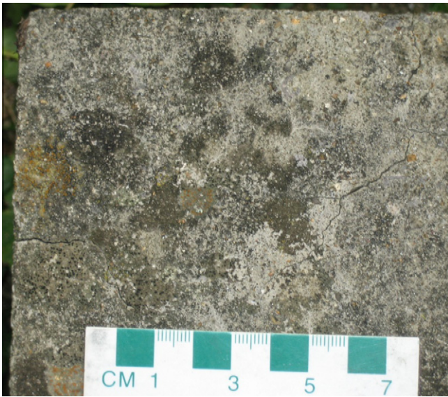
Fig. 9. Fine cracking on 350-mm block with 450 kg/m 3 PC and 150 kg/m 3 DX fly ash at 17 years.
