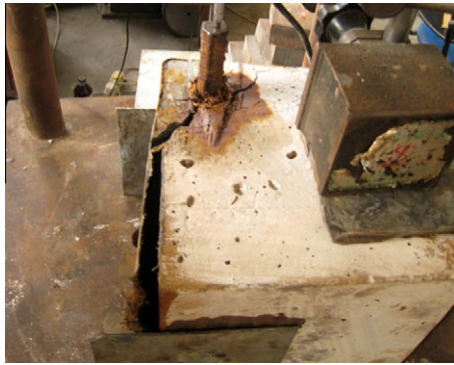
Fig. 5. CFRP sheets peeling off during splitting failure of specimen 25-R15.
