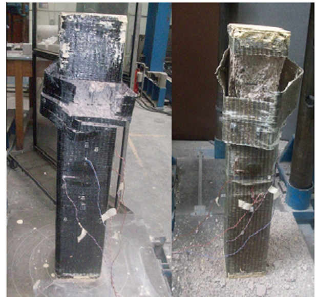
Fig. 4. Failure pattern of FRP composites.
