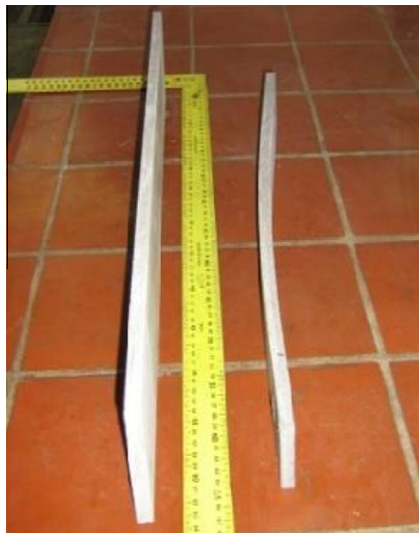
Fig. 5. Illustration to the effect of the production technique on the shrinkage of the specimens: a specimen made by casting in two moulds subsequently pressed together (left side), and a specimen cast in one piece (right side).
