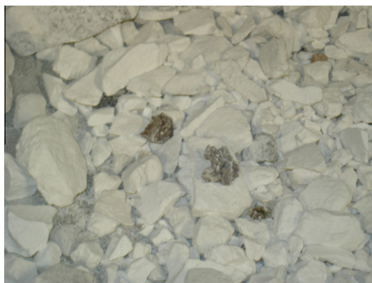
Fig. 1. Darker impurities in the industrial quicklime in stone.
