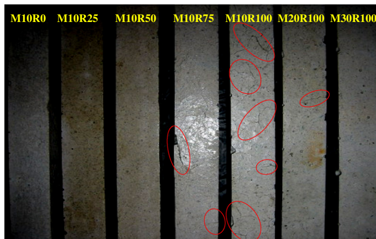
Fig. 7. ASR cracks of RG-SCWM bars after 28 days storage in 1 N NaOH at 80 °C.
