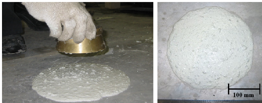
Fig. 1. Mini-slump flow test for RG-SCWM.
