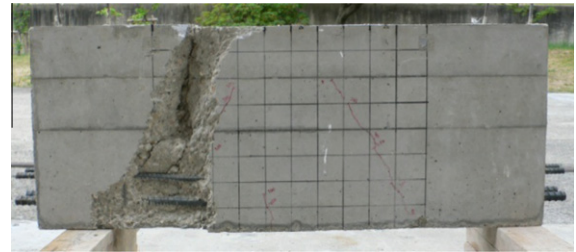
Fig. 21. Failure of BS4bw100.
