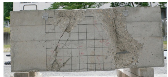
Fig. 22. Failure of BS4bw200.
