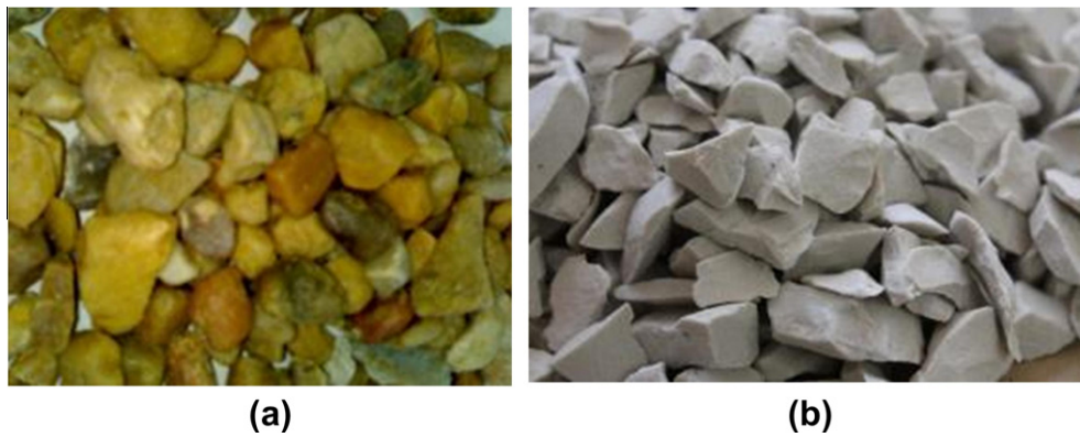
Fig. 1. Illustration of (a) natural gravel aggregate and (b) recycled ceramic aggregate.
