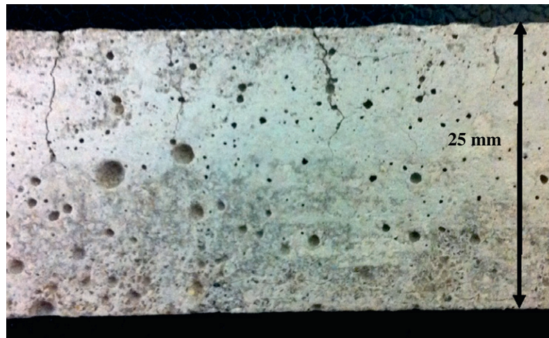
Fig. 14. Typical one-sided cracking of the 25 × 25 × 280 mm bars, responsible for non-symmetric ionic diffusion.
