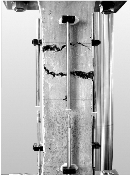
Fig. 5. Example of crack patterns obtained at the end of the tensile test.
