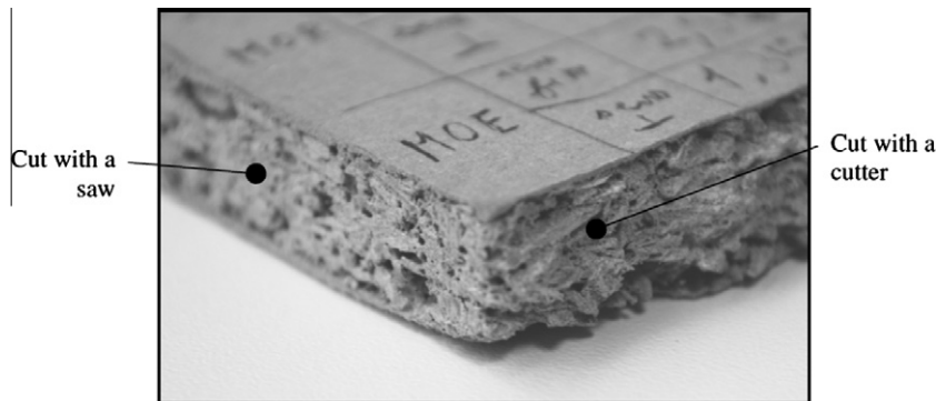
Fig. 3. Front of rupture of a wood–cement particleboard cut with a knife (on the right side of the photo; the other side was cut with a saw).
