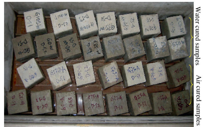
Fig. 13. Appearance of water on the top surface of water and air cured SCGC specimens after exposure to 800 °C and 4 h of water sorptivity test. Note: The labels on each sample represent: Gxx (glass content), A or W (air or water cured), D (800 °C) and Sx (sample number).
