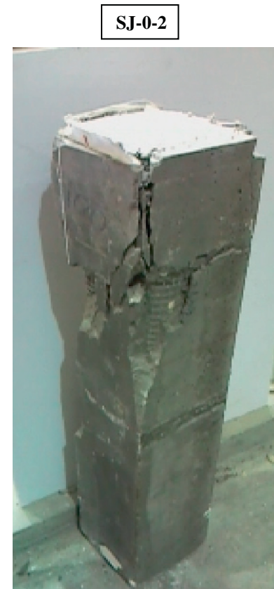
Fig. 7. Typical failure mode for jacketed column specimens without preloading.
