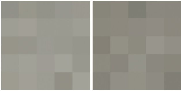
Fig. 9. Lab matrices of w/c 0.45 untreated (left) and treated (right) samples, at the end of the curing.
