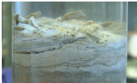
Fig. 4. Layer of deteriorated TSA affected concrete, 27 months.
