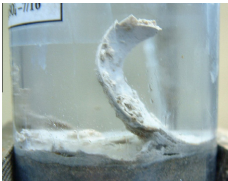
Fig. 3. Carbonated crust, 9 months.
