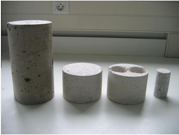
Fig. 2. Coring of 4 × 8 cm cylinders from 11 × 22 cm cylindrical concrete specimens.
