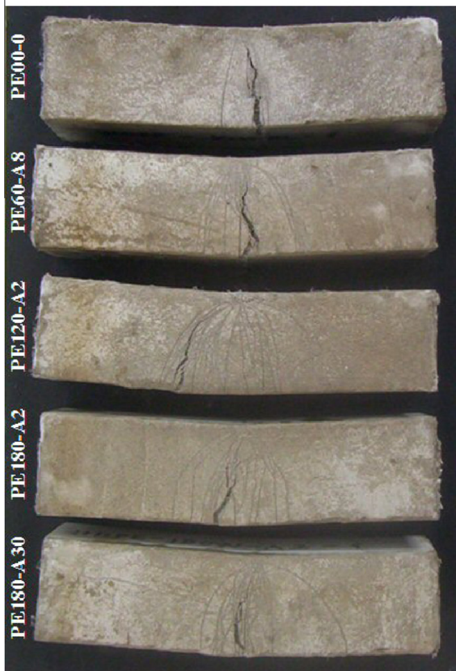
Fig. 9. The load–deflection curves and photographs of PE fiber reinforced unnotched composites at 28 days: (a and c) incorporating argon plasma treated fibers, (b and d) incorporating oxygen plasma treated fibers.
