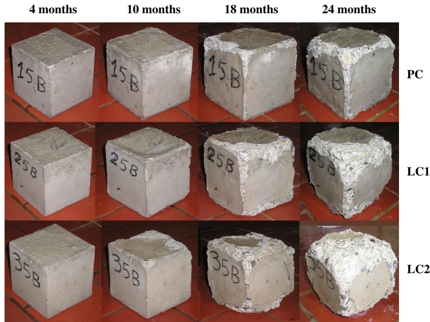
Fig. 4. Concrete specimens after 4, 10, 18 and 24 months of exposure in S solution.
