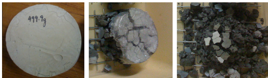
Fig. 4. OPC paste 800 °C. Left, after 800 °C heat treatment. Middle, immediately after water immersion. Right, few minutes after water immersion.
