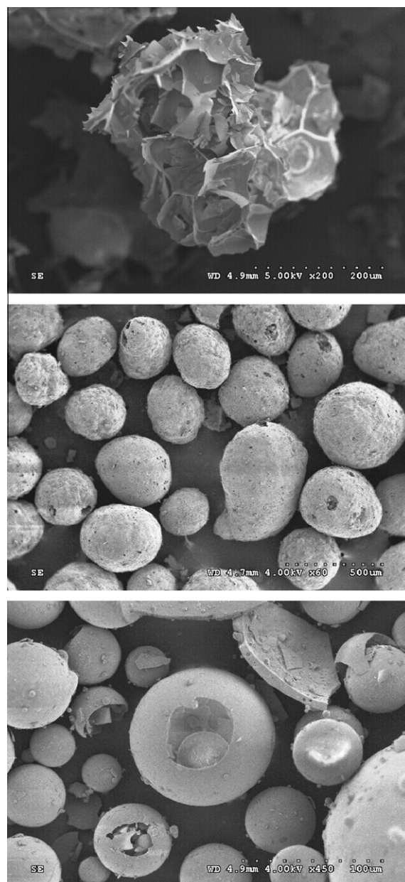
Fig. 1. SEM images showing the morphology of expanded perlite (top); expanded glass (middle) and cenospheres (bottom).
