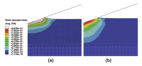
Fig. 8. Effect of contact friction on the extent of the plastic zone. (a) LD C-S-H with  $\mu$  = 0 (sample A0) and (b) LD C-S-H with  $\mu$  = 0.25 (sample A2).
