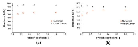
Fig. 7. Hardness values of the (a) LD C-S-H and (b) HD C-S-H, as calculated using the Oliver and Pharr and numerical methods for various friction coefficients.
