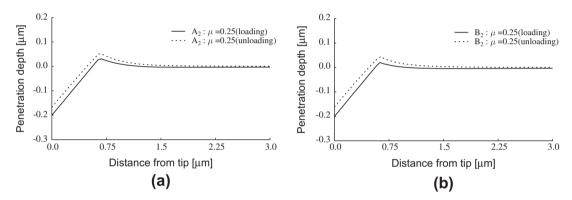
**Fig. 9.** Displacement profiles in the loaded and unloaded configuration. (a) LD C–S–H with  $\mu$  = 0.25 (sample A2) and (b) HD C–S–H with  $\mu$  = 0.25 (sample B2). The projected area of contact remains unaffected.
