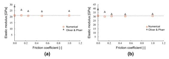
Fig. 6. Elastic moduli of (a) LD C-S-H and (b) HD C-S-H, as calculated using area estimations of the Oliver and Pharr and numerical methods, for various friction coefficients.
