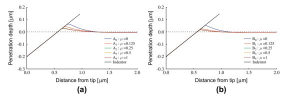
Fig. 3. Deformation profiles of the LD and HD C-S-H. A maximum depth of 200 nm is used.
