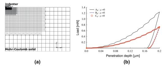
Fig. 1. (a) Geometrical details and finite element mesh of the studied problem. (b) Resulting force versus penetration depth curves of simulated indentation on the three model materials, frictionless LD (A0), HD C-S-H (B0) and a model material (C0).
