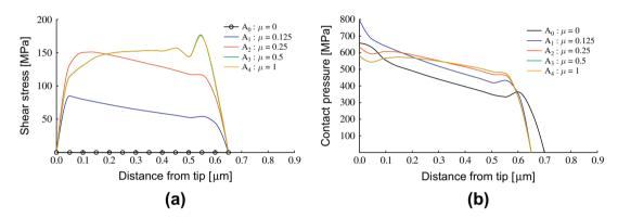
Fig. 4. Effect of contact friction on the distribution of (a) contact shear stress and (b) contact pressure for the LD C-S-H (samples of series A).
