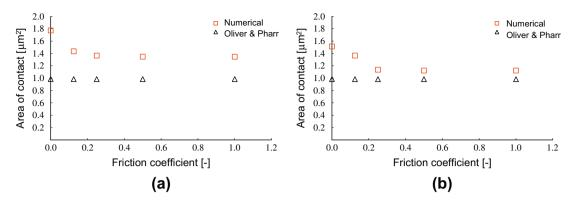
Fig. 5. Area of contact as obtained using the Oliver and Pharr method and numerical techniques for (a) LD C-S-H and (b) HD C-S-H.
