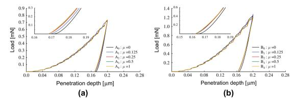
Fig. 2. Effect of contact friction on the simulated indentation force versus penetration depth (P-h responses) of LD and HD C-S-H.
