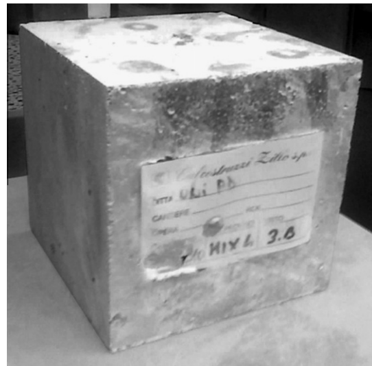
Fig. 3. White powder outcrops on specimens after accelerated ageing treatment.
