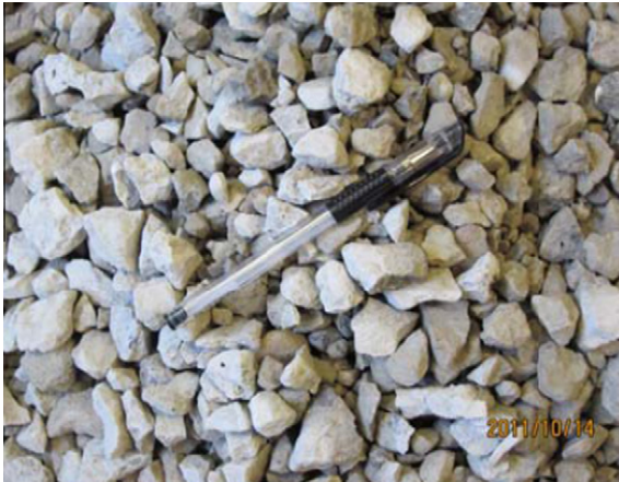
Fig. 1. Recycled coarse aggregate (4.75–25.0 mm) (Rossi Contractors Inc. in Chicago, IL).
