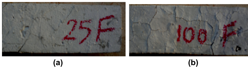
Fig. 10. Cracking in (a) 25F and (b) 100F specimens.
