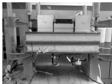
Fig. 2. Thermal conductivity (guarded plates) test setup (two 20 \times 300 \times 300\text{ mm} plates).
