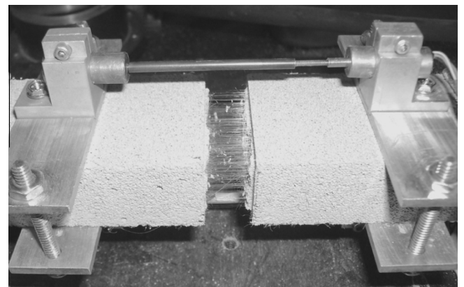
Fig. 17. Crack bridging for notched FRAC-A prism during tensile test.
