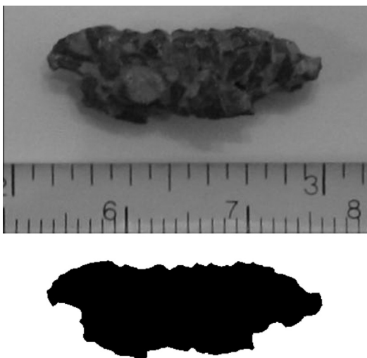
Fig. 9. Post-failure fragment and its maximum projected profile.
