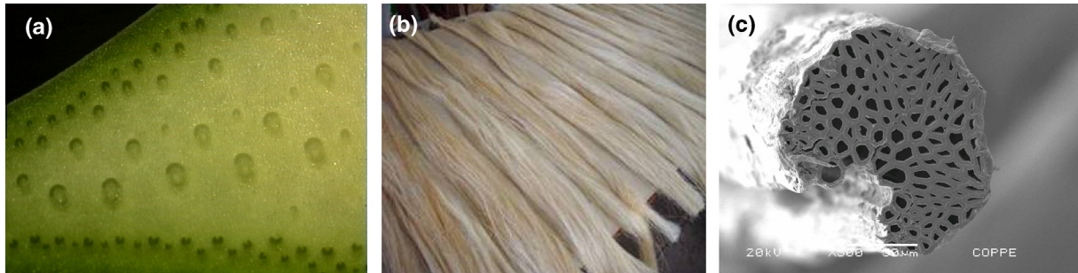
Fig. 1. The sisal plant and its fiber: (a) a sisal leaf showing the sisal fiber distribution, (b) the fiber after being extracted and cleaned and (c) the microstructure of the sisal fiber which is formed by several fiber-cells.
