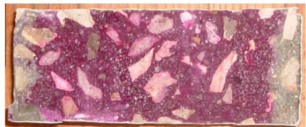
Fig. 1. Cross-section of a split core with carbonation fronts from natural carbonation (left-hand side) and accelerated carbonation (right-hand side).
