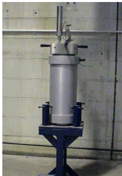
Fig. 2. Photo and diagram illustrating the \text{scCO}_2 reaction vessel.
