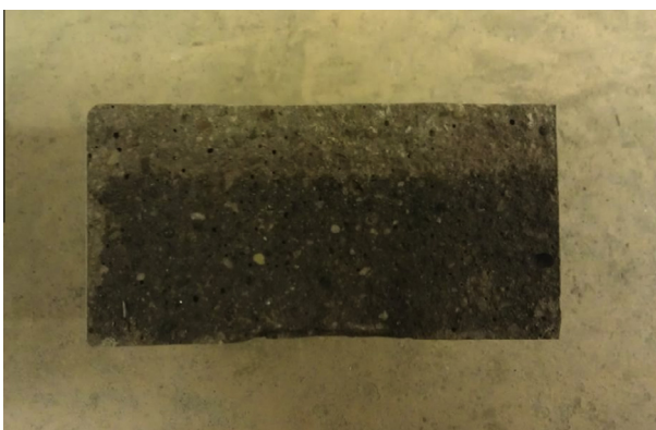
Fig. 2. A sample from the rapid chloride migration (RCM) test that was split and sprayed with silver nitrate ( \text{AgNO}_3 ).
