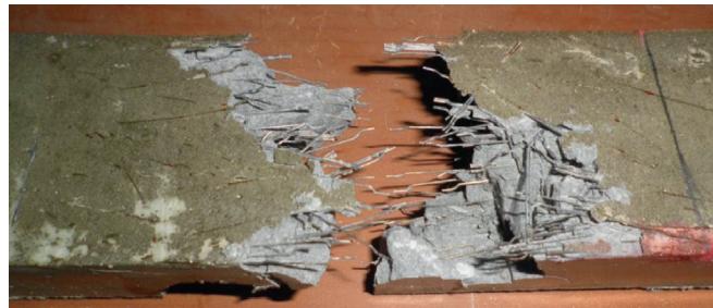
(b) The fibers of H-specimens almost still remain the hooks in static test
