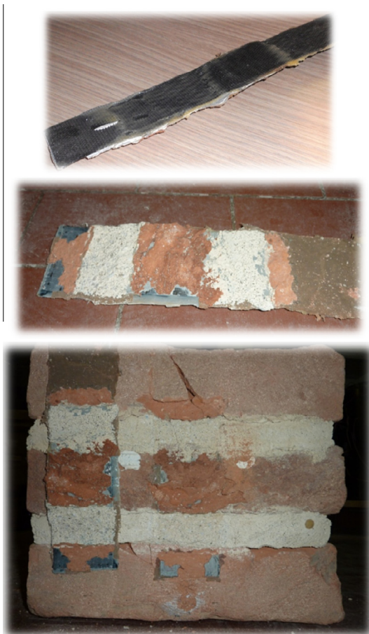
Fig. 12. Post-mortem pictures of masonry pillar and detached reinforcement. Part of the support is still glued to the CFRP strip, thicker in the middle (over the second brick), and indicates the bulk collapse mechanism.
