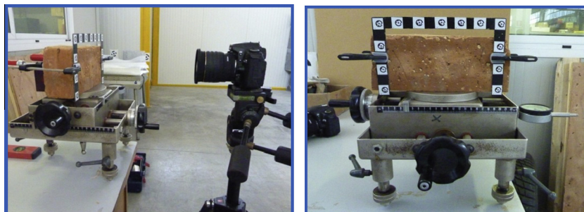
Fig. 4. Validation of optical monitoring system in the laboratory, by means of a dual-axis slide (with accuracy \pm 10 \mu\text{m} ) and a registration frame with control points.
