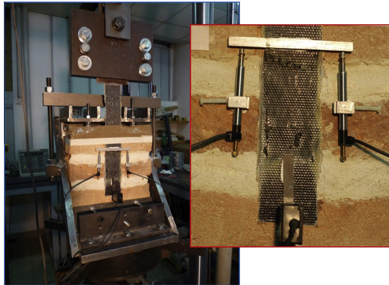
Fig. 2. The testing frame stiffened by diagonal connecting rods, including the reinforced masonry pillar. In the close-up window a detail of the monitored surface is shown, equipped with two LVDTs and a clip gauge.
