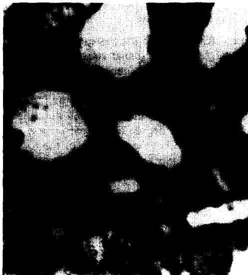
Fig. 9 BSE image for slag paste activated with NaOH at 1 year, showing clearly the "rims" around slag particles and their darker appearance than "general" products.
