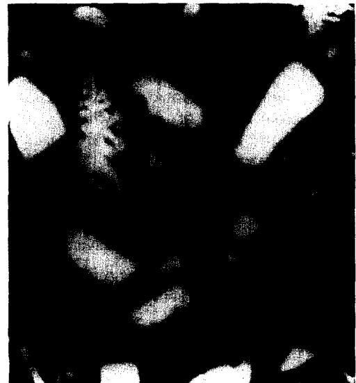
Fig. 10 BSE image for slag paste activated with waterglass at 1 year, showing clearly the "rims" around slag particles and their darker appearance than "general" products.
