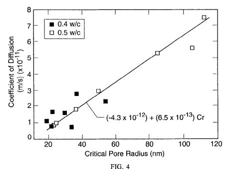
Chloride diffusion coefficient vs. critical pore radius (Cr) for portland cement pastes and mortars.
