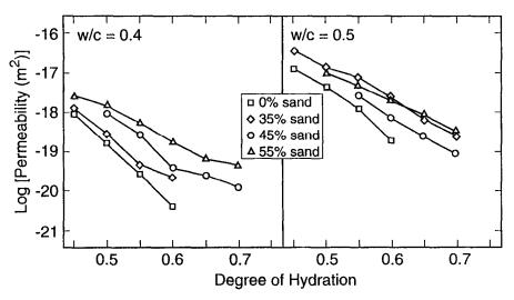
FIG. 3 Permeability vs. degree of hydration for 0.4 and 0.5 w/c ratio mixes.
