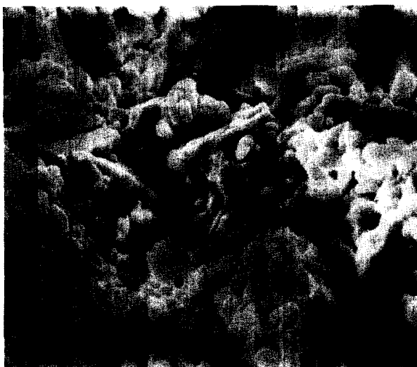
FIG. 4.- SEM Micrograph of J Mortar (P Group) (x3000)
