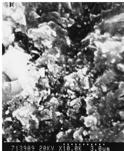
FIG. 1. SEM image of hydrated plain cement paste.
