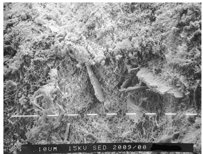
Fig. 3. Hydration products near the primer layer in EP/UN samples.
