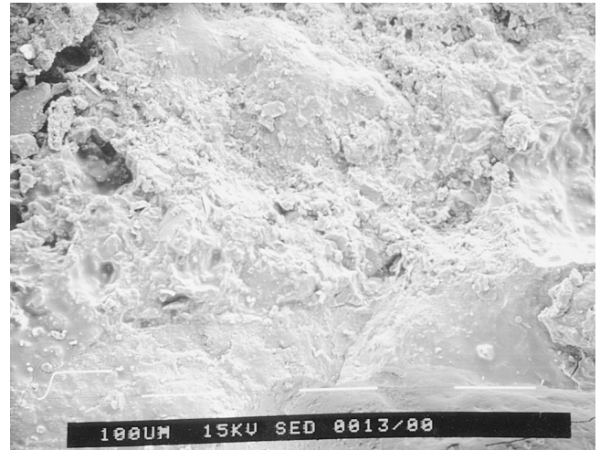
Fig. 2. Microstructure of the EP/EP system: substrate (bottom) and repair mortar (top).
