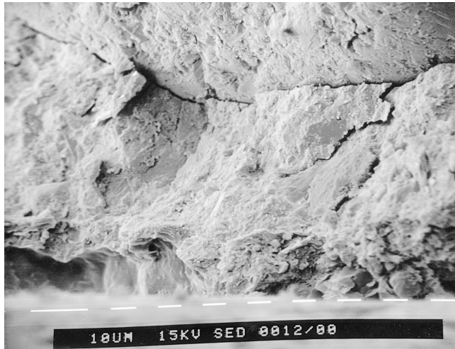
Fig. 4. Microcracks in the substrate of an EP/UN sample submitted to thermal cycle 2.
