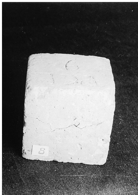
Fig. 14. Concrete cube having polyurethane-coated MS rebars (80 cycles).
