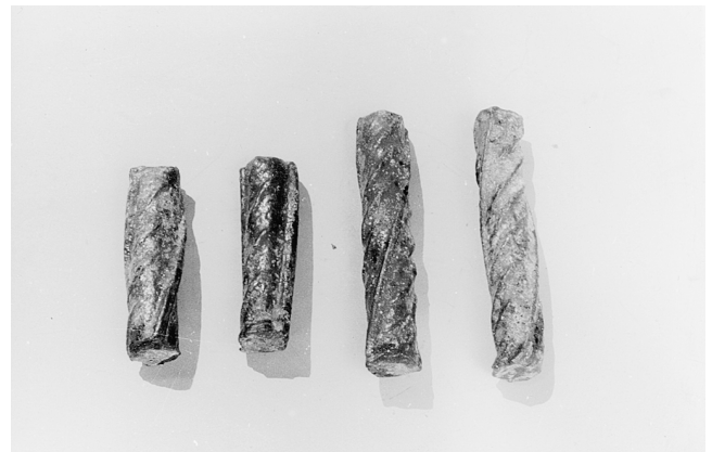
Fig. 20. Condition of fusion-bonded epoxy-coated rebars after 60 cycles.
