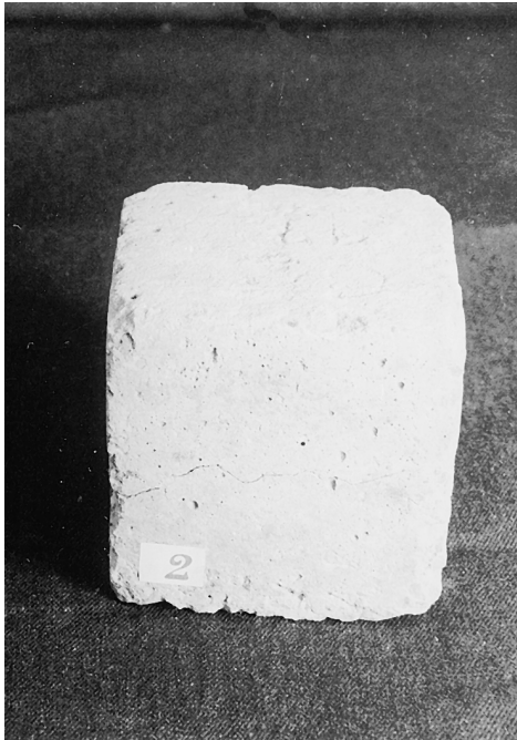
Fig. 10. Concrete cube having uncoated CRS rebars (50 cycles).
