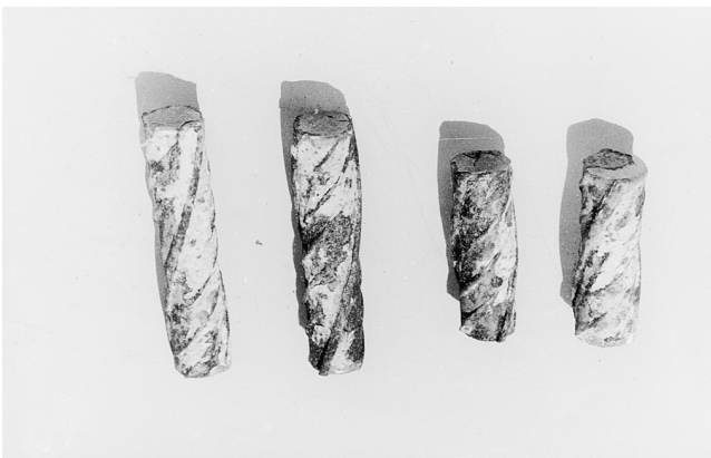
Fig. 19. Condition of IPN-coated rebars after 60 cycles.
