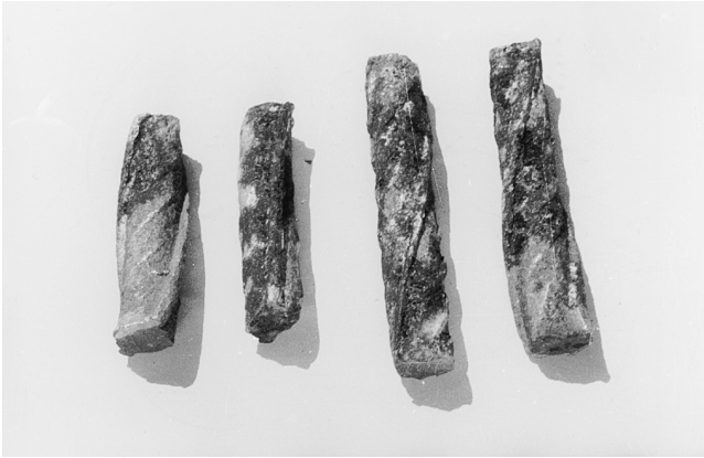
Fig. 18. Condition of MS uncoated rebars after 60 cycles.
