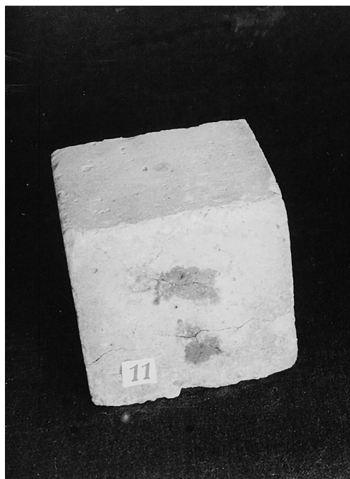
Fig. 17. Concrete cube having fusion-bonded epoxy-coated rebars (80 cycle).
