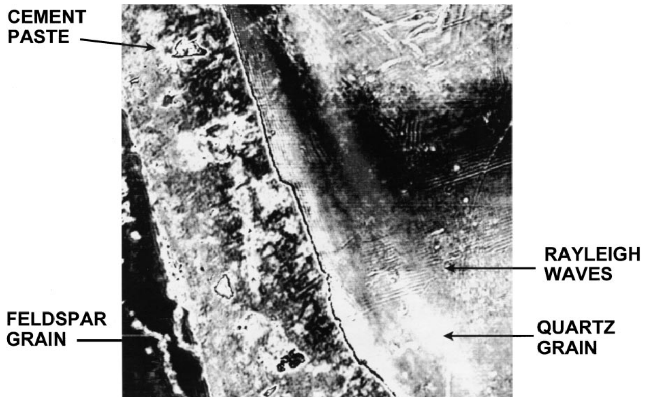
Fig. 3. SAM image of interfaces among cement matrix and aggregate grains. Image size is 1000 \times 1000 \mu\text{m} .
