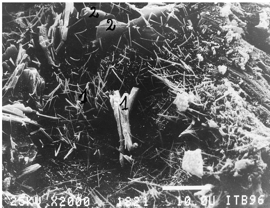
Fig. 4. SEM image of concrete with SMF superplasticizer, 200 cycles of freezing and thawing (magnification 2000 \times ). 1, ettringite; 2, hydrated calcium aluminates.
