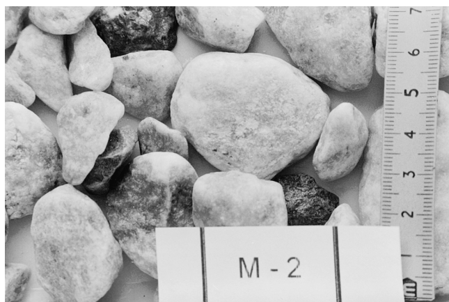
Fig. 2. Gypsum 2. Massive gypsum with greater crystal size than in Figure 1.
