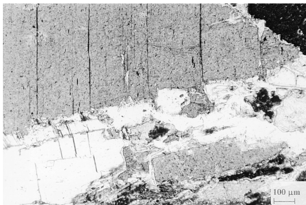
Fig. 8. Gypsum 2. Gypsum replaces anhydrite; both show big grain sizes and marked cleavage systems.
