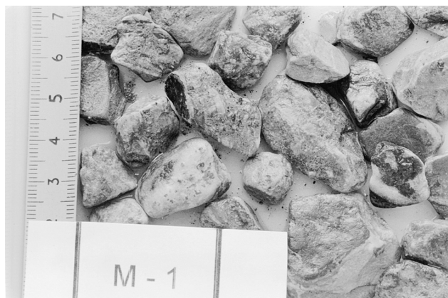
Fig. 1. Gypsum 1, with predominant sedimentary structures. It can be seen that some fragments have a brecciated aspect.
