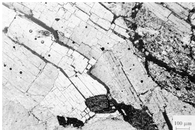
Fig. 10. Gypsum 2. Big grains of gypsum and anhydrite. The strong cleavage makes breakage easier.
