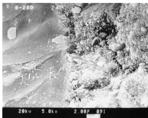
Fig. 7. SEM of expansive concrete paste-aggregate under confined-curing condition.
