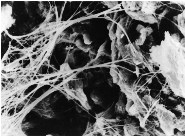
Fig. 4. SEM micrograph (mag. \times 2000 ) of 1L 5S sample after exposure to deionised water for 28 days.
