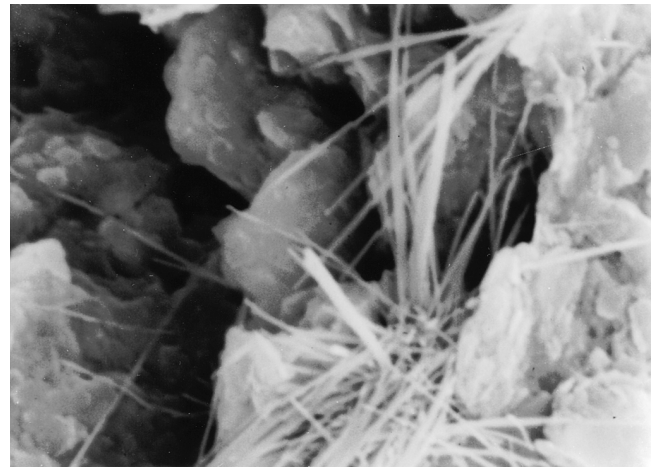
Fig. 2. SEM micrograph (mag. \times 2000 ) of 3L 3S after exposure to \text{Na}_2\text{SO}_4 solution for 7 days.
