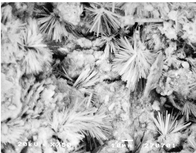
Fig. 5. SEM micrograph of 0L 6S sample after exposure to \text{Na}_2\text{SO}_4 solution for 28 days.
