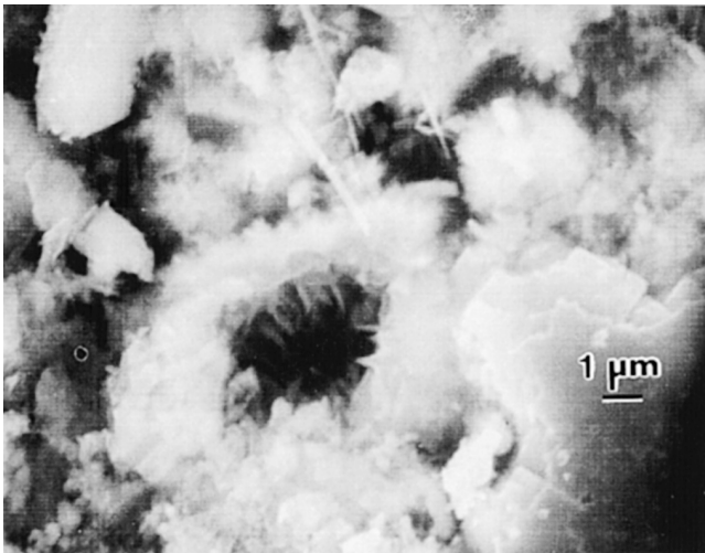
Fig. 4. Paste side of 3-day-old 0.5 water:cement specimen showing hollow-shell grain in center. Note portion of duplex film carried with paste, lower right corner.
