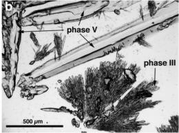
Fig. 2. Micrograph of thenardite crystals. (a) Precipitated at 20°C and low RH conditions (>40%); the needles are phase III and the prisms are phase V crystals [37]. (b) Large phase V bipyramidal prisms precipitated at 20°C and 13% RH. Small amounts of phase III needles are also present.
