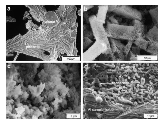
Fig. 4. Sodium sulfate ESEM micrographs. (a) Thenardite crystals precipitated on glass slides. (b) Thenardite aggregates formed after dehydration of preexisting mirabilite crystals (ESEM dynamic study). (c) Detail of thenardite crystals formed after dehydration of mirabilite. (d) Thenardite crystals precipitated directly from solution on the Al sample holder in the ESEM.
