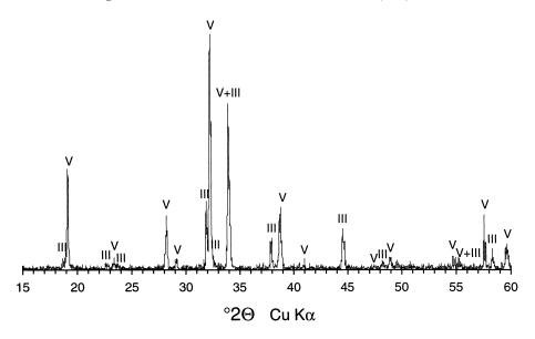
Fig. 3. The XRD pattern of thenardite (phases III and V) precipitated directly from solution at  $20^{\circ}$ C and RH <40%.
