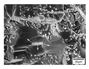
Fig. 5. Thenardite on the underside of a decayed limestone spall fragment. Note the similarity of these crystals with the thenardite crystals precipitated in the ESEM chamber (Fig. 4d).
