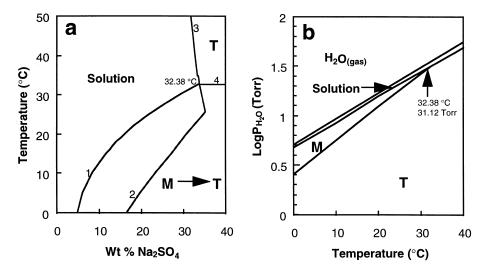
Fig. 1. The system,  $Na_2SO_4-H_2O$ . (a) Temperature vs. concentration diagram (M=mirabilite; T=thenardite; 1=solubility curve for  $Na_2SO_4\cdot10H_2O$ ; 2=solubility curve for  $Na_2SO_4\cdot10H_2O$  boundary). (b) P/T phase diagram for the system,  $Na_2SO_4-H_2O$ . Data sources: Refs. [16,19,20].
