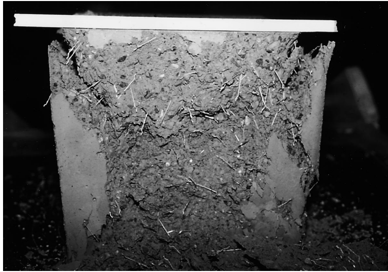
Fig. 2. Steel fibre distribution in the cube of SFRC after the test of compression strength.
