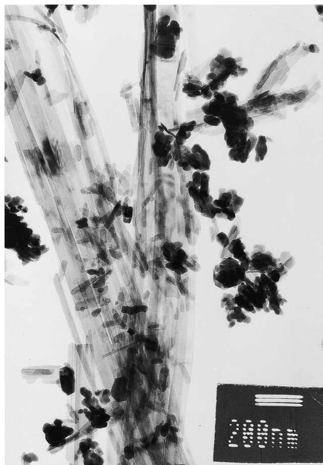
Fig. 2. TEM micrograph of \text{Ca}_2\text{Ce}_8(\text{SiO}_4)_6\text{O}_2 (platelets and prisms) and C–S–H impurity (laths and needles).
