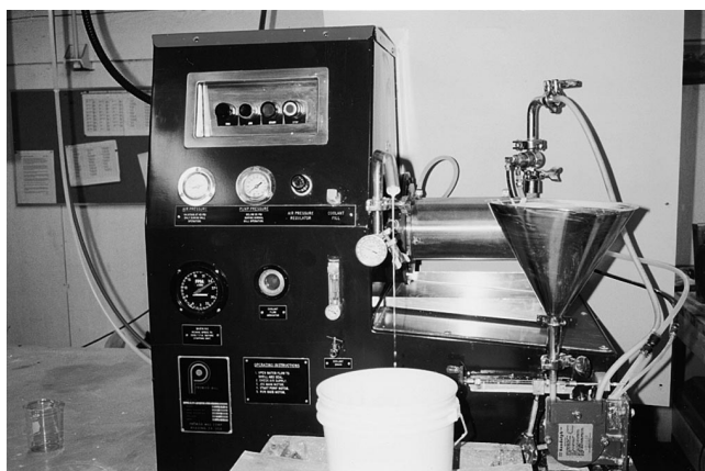
Fig. 2. Illustration of the agitated ball mill-grinding machine.
