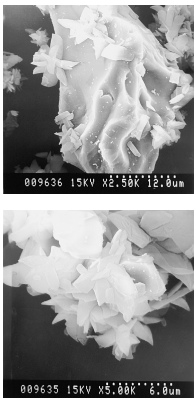
Fig. 8. Development of struvite crystals.
