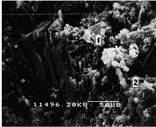
Fig. 1. SEM micrograph of unmodified mortar. 2800 × 2K; Arrow 1: large crystal; Arrow 2: large pore.
